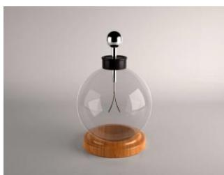
A gold leaf electroscope measures potential difference between the leaf and the base (or earth).
